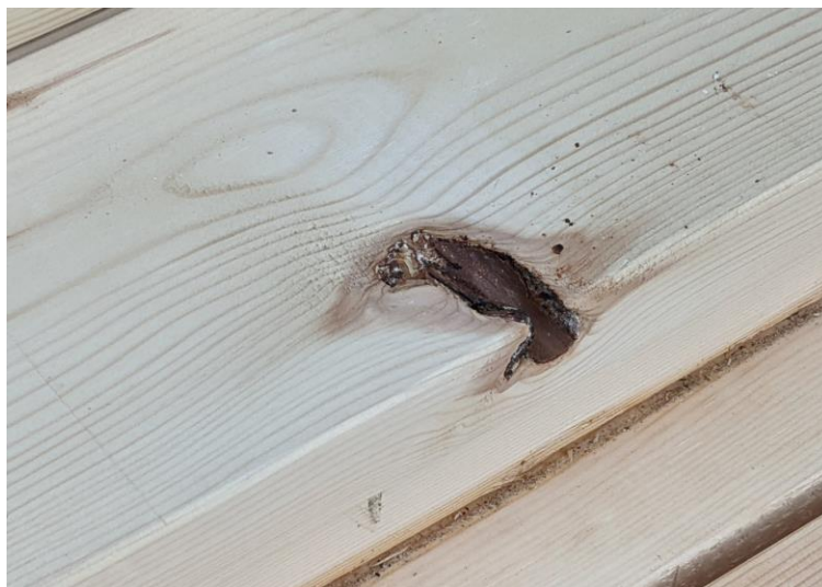
A Slough knot hole running from one wide face into the adjoining narrow face
