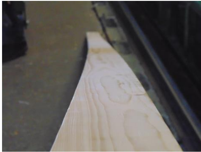
Crook deviation looking down a board
