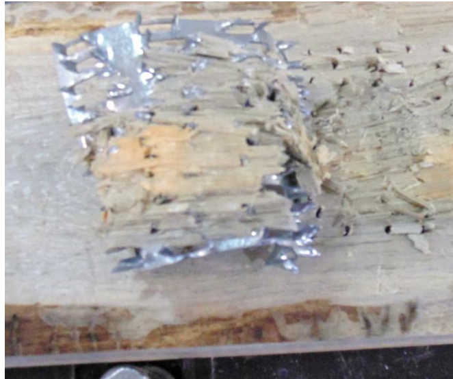
Plate removal with fiber tear-out usually with air chisel
