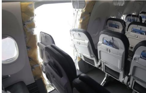
Boeing door plug that was missing 4 bolts
