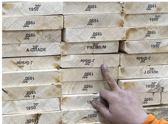
Wrong grade of lumber in a lift
